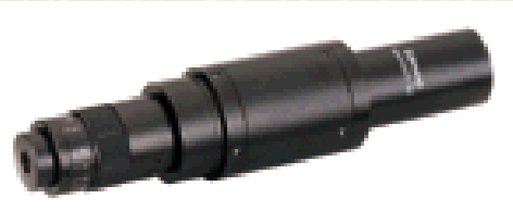
Edmund VZM1000 FOV 0.64-2.5mm on 1/2" CCD Zoom x2.5-10 Space Resolution max. 228lp/mm (4.4micron)
